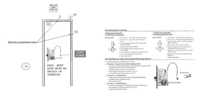
EXISTING FRAMES - WILL BE USING SS WIRE LOOP TO TRANSFER WIRE FROM WALL TO DOOR. NEW FRAMES TO HAVE WIRE PRE-INSTALLED BEFORE DELIVERY TO SITE.
