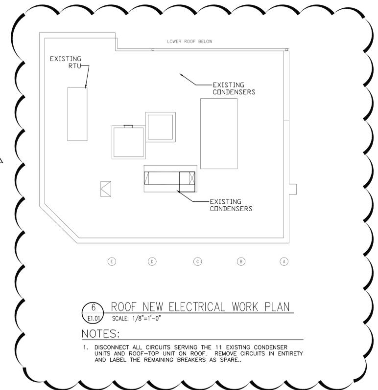
**6 ROOF NEW ELECTRICAL WORK PLAN**
